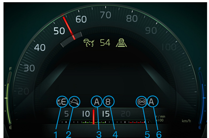
Shown on the display: 1. Drive mode 2. I-See symbol (Green = Working / Grey = Engaged “Ready to work”) 3. Automatic gear shifts / Manual gear shifts 4. Selected gear 5. Aux Brakes engaged 6. Brake level in position automatic (A=Brake blend)
