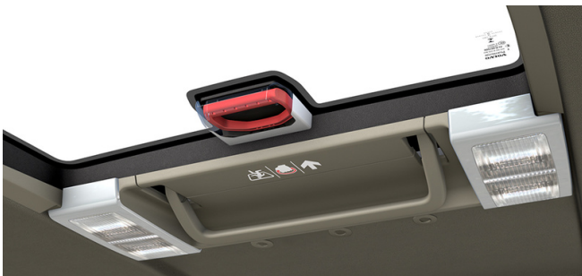
Emergency handle for Volvo FM/FH laminated glass sky window and roof hatch.
