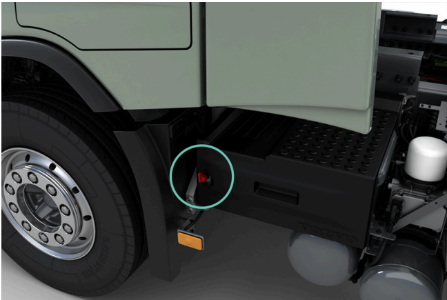
Chassis-installed main switch for BATS-S (BBOX-L).
