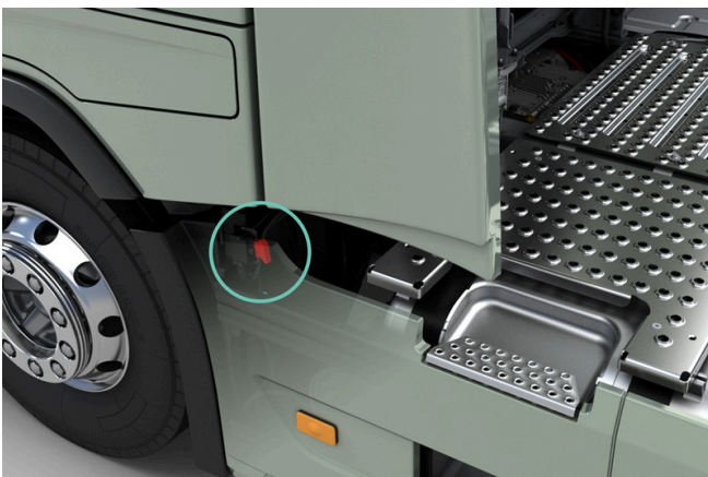
Chassis-installed main switch for BATS-S (BBOX-EF).
