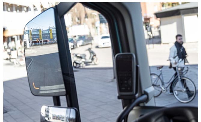
A static light in the rear-view mirror informs the driver that an object is detected on the side of the vehicle.
