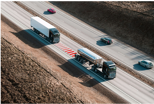
Adaptive Cruise Control adapts and maintains the selected distance to the vehicle ahead.
