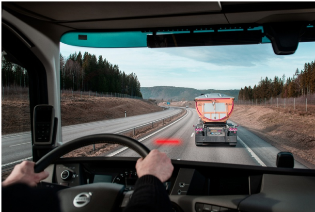
Forward Collision Warning with a red light signal reflected in the windscreen.
