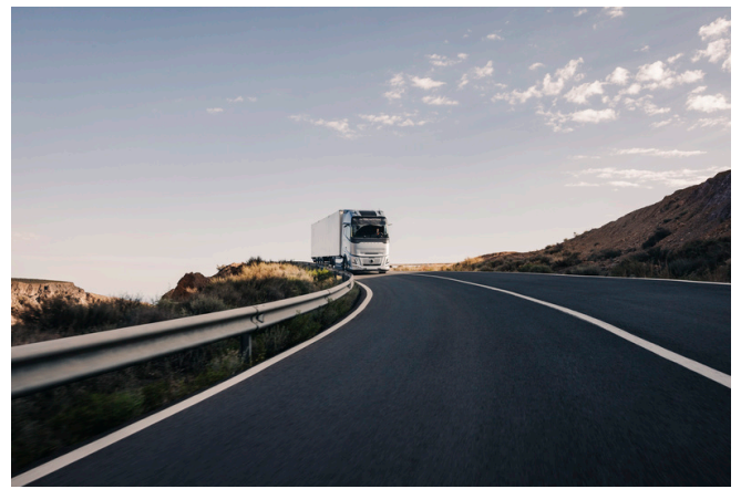
Stability Assist helps the driver keep control of the truck by adding a guiding steering torque when the trucks start to skid.
