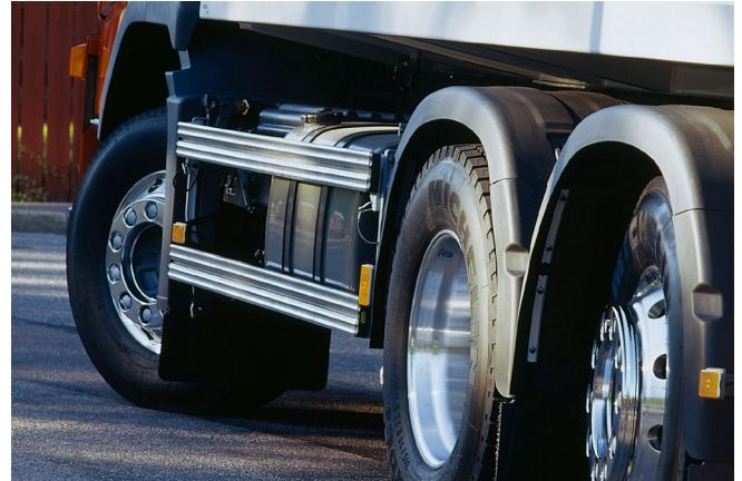
Left hand mounted fuel tank in steel.
