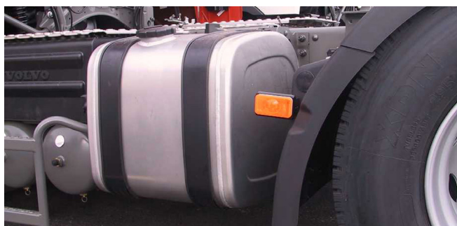
Left hand mounted fuel tank in aluminium.
