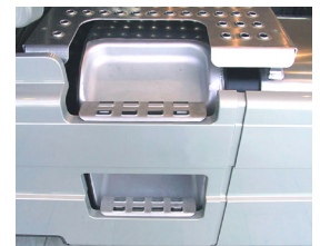
Steps with a non-skid perforation in AD-CHASX.
