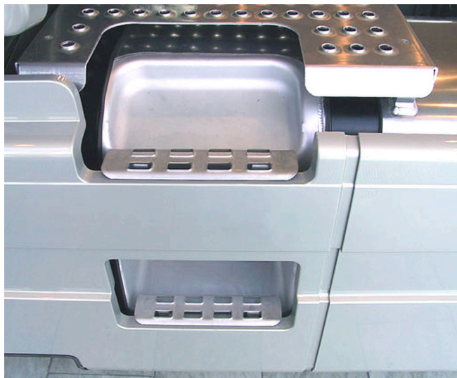
Steps with a non-skid perforation in AD-CHASX.
