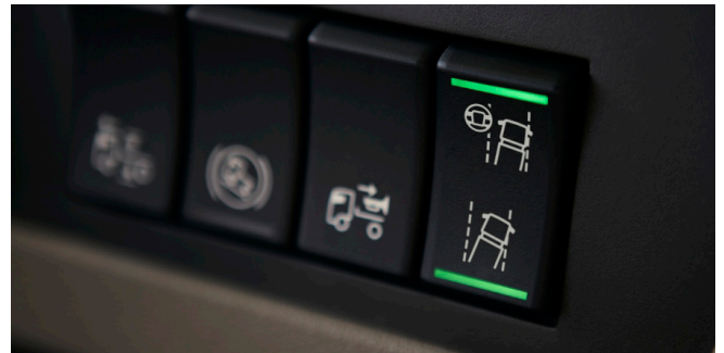
The functions in Lane Keeping Assist are handled with a switch on the instrumental panel.
