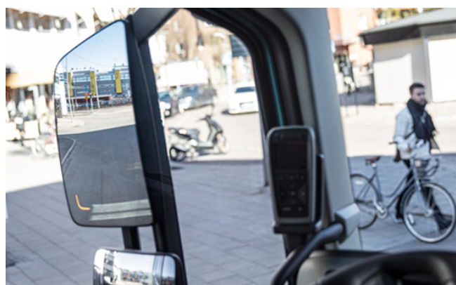
A static light in the rear-view mirror informs the driver that an object is detected on the side of the vehicle.
