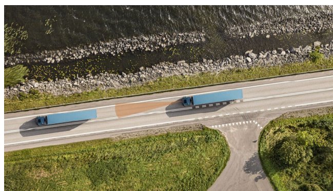
The Lane Keeping Assist uses a front-facing camera to track the lane markers. When the truck is on its way to cross the line, the system supports the driver with a gentle Steering to come back to the middle of the lane again.
