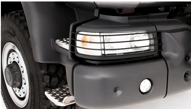
Non-slip footsteps in steel and headlamps with optional protection.
