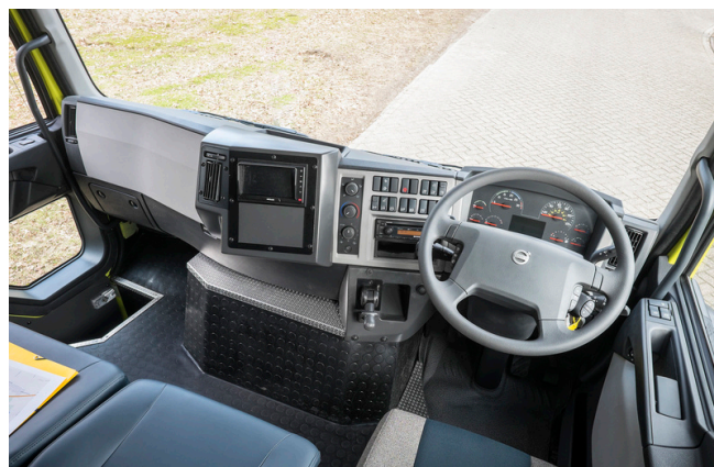
Separate console for parking brake, when specified with AT2412F, including small storage space. Note! Dual double DIN adapter in dashboard according to S90150. Monitor not included in this option. Picture showing STWPOS-R.
