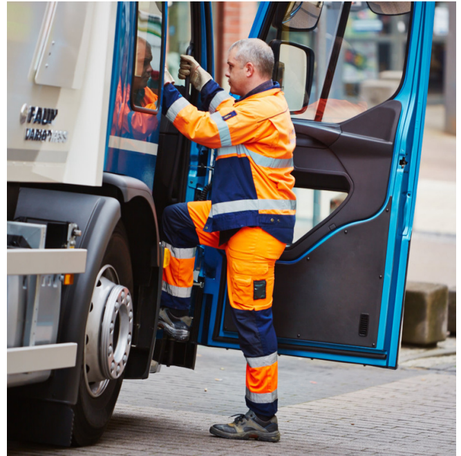
Low and ergonomic instep with kneeling function and 90-degree door opening. Picture showing STWPOS-L.
