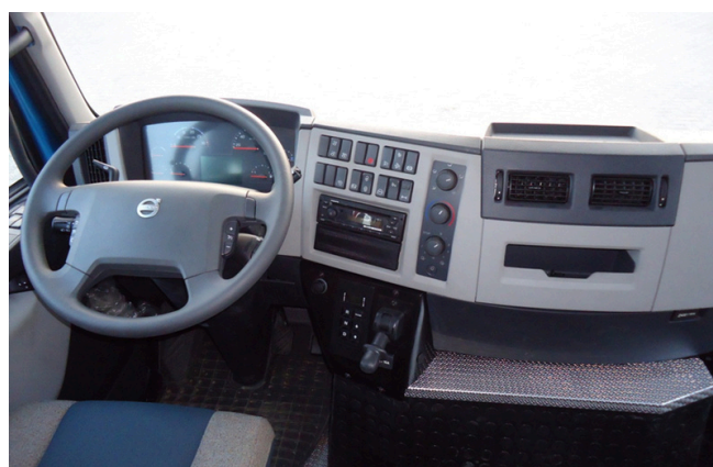
Standard dashboard, but slightly modified due to LEC conversion. Separate console for parking brake and AL306 controls. Picture showing STWPOS-L.
