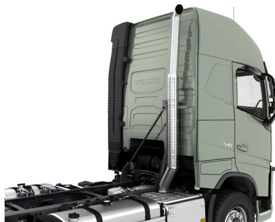
Vertical exhaust top pipe in bright polished stainless steel (EXST-SSP)
