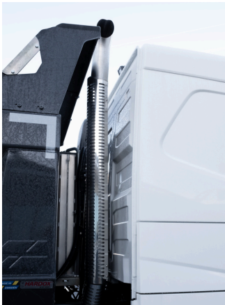
Vertical exhaust top pipe in aluminised steel (EXST-ST)
