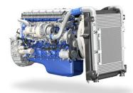
The D8K350, EU6SCR is an in-line six-cylinder diesel engine with a displacement of 7.7 litres, equipped with a turbocharger and intercooler. The engine produces 350 hp and 1400 Nm of torque. The engine meets the EU exhaust emissions requirements according to the Euro 6 standards.
