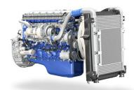
The D8K320, EU6SCR is an in-line six-cylinder diesel engine with a displacement of 7.7 litres, equipped with a turbocharger and intercooler. The engine produces 320 hp and 1200 Nm of torque. The engine meets the EU exhaust emissions requirements according to the Euro 6 standards.
