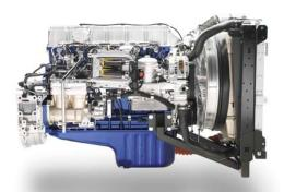
The D7F240 is an in-line six-cylinder diesel engine with a displacement of 7.2 litres, equipped with a turbocharger and Intercooler. The engine produces 240 hp and 940 Nm of torque. The engine meets the EU exhaust emissions requirements according to the Euro 5 standards.
