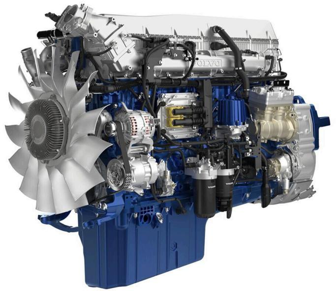
The D17A780 is a 780 hp with 3800 Nm, 17.3 litres, in-line, six-cylinder diesel engine. Equipped with an overhead camshaft, four valves per cylinder, common rail fuel injection and an efficient variable geometry turbo (VGT). The engine is very fuel-efficient and meets the Euro 6 exhaust emissions requirements.
