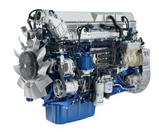
The D13K540 is a 540 hp, 12.8-litre, in-line, six-cylinder diesel engine equipped with an overhead camshaft, four valves per cylinder and common rail fuel injection. The engine meets the Euro 6 exhaust emissions requirements.
