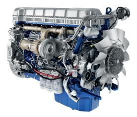
The D13K460 is a 460 hp, 12.8-litre, in-line, six-cylinder diesel engine equipped with an overhead camshaft, four valves per cylinder and common rail fuel injection. The engine meets the Euro 6 exhaust emissions requirements.
