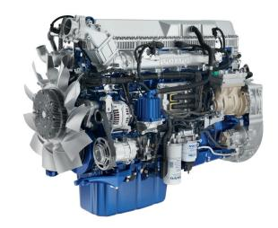
The D13K460 is a 460 hp, 12.8-litre, in-line, six-cylinder diesel engine equipped with an overhead camshaft, four valves per cylinder and common rail fuel injection. The engine meets the Euro 6 exhaust emissions requirements.
