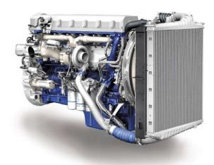
The D13C460 is a 460 hp 12.8-litre in-line, six-cylinder diesel engine equipped with an overhead camshaft, four valves per cylinder and unit injectors. The engine meets the EU exhaust emissions requirements according to the Euro 5 standards.
