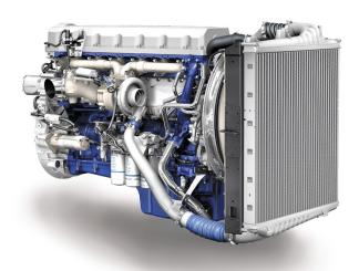
The D13A540 is a 540 hp 12.8-litre in-line, six-cylinder diesel engine equipped with an overhead camshaft, four valves per cylinder and unit injectors. The engine meets the EU exhaust emissions requirements according to the Euro 4 standards.
