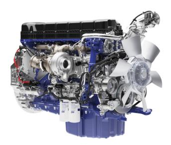
The D11S460A is a 460 hp, 10.8 litres, in-line, six-cylinder diesel engine equipped with an overhead camshaft, four valves per cylinder and common rail fuel injection. The engine meets the Euro 6 exhaust emissions requirements.
