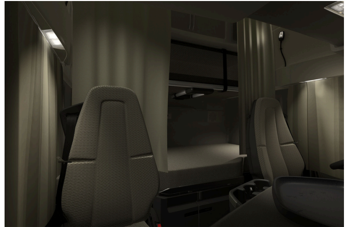
Example of curtain installation for curtains between seats and beds. Note that the colour pattern can differ between Volvo FM and Volvo FH.
