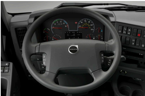
Activation and setting of speed are done with buttons on the steering wheel.
