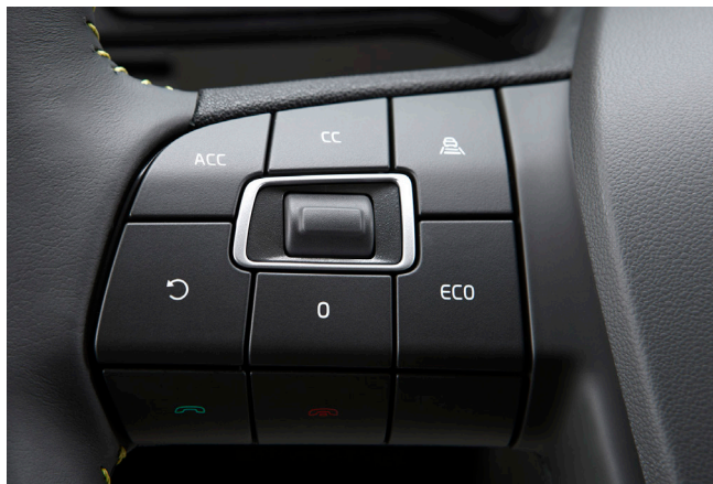
Buttons for CRUIS-E cruise control in the steering wheel. ECO-button to the right. Eco level will be set with the scroll wheel in the middle.
