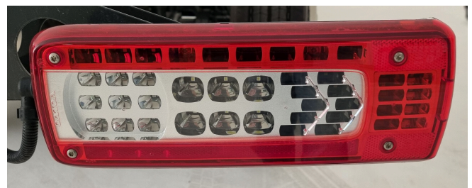
Tail lights with integrated reversing warning unit.
