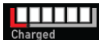
The white boxes representing how much the battery are charged. The red area representing the reserve of energy needed to start the engine.
