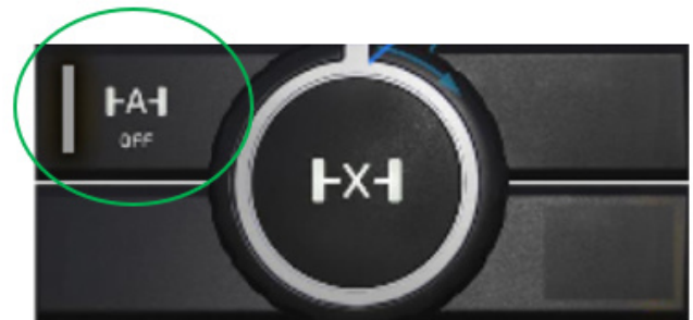
When the indicator is not lit, the automatic differential locking (A) is activated.
