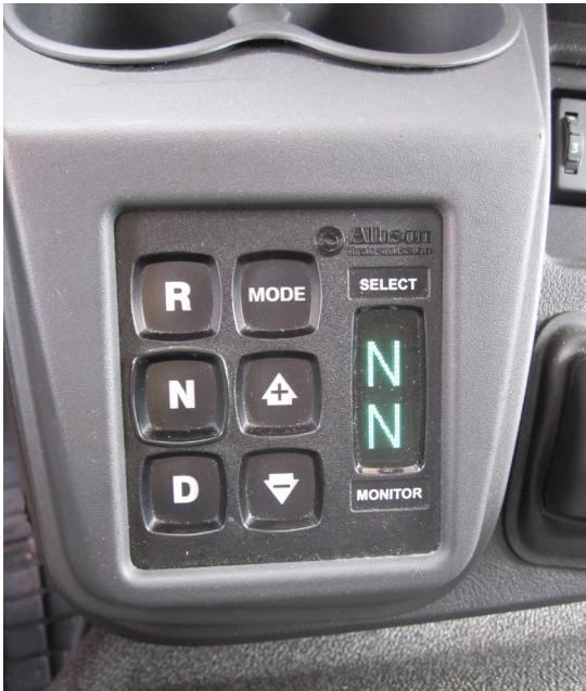
Push-buttons shift selector – Volvo FL.
