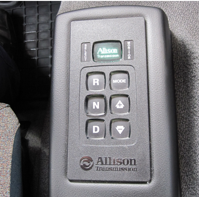
Push-buttons shift selector – Volvo FE.
