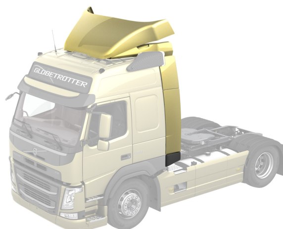
FM-HSLP, AD-SIDES, AD-ROOF altura alta
